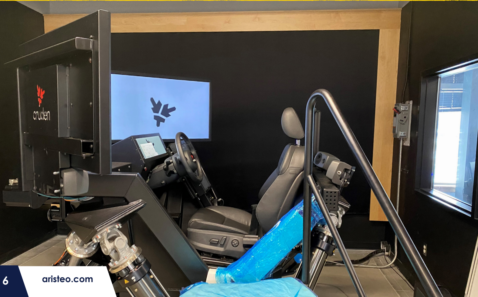
Aristeo sourced and installed a custom wood valance system to eliminate the risk of natural light affecting the simulator.
